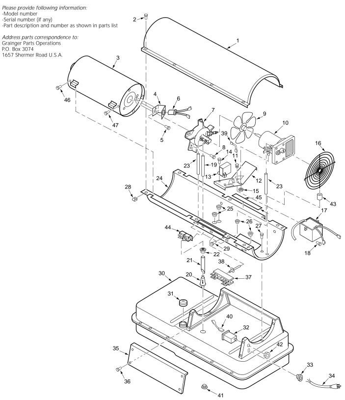
Figure 24 - Replacement Parts Illustration for Model 3VG79
